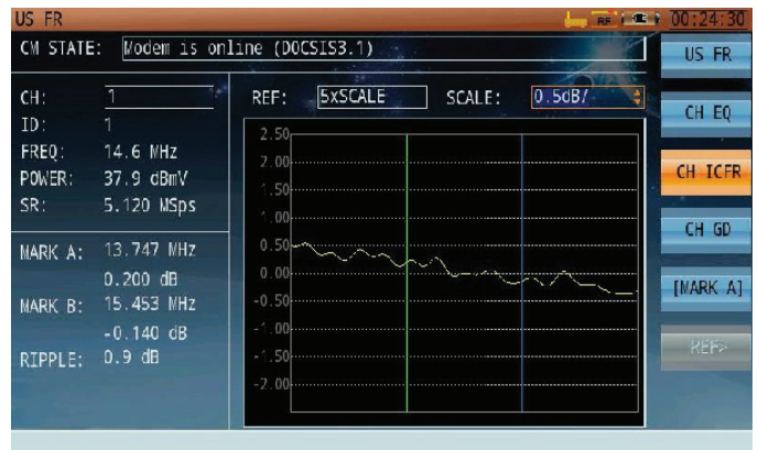
Figure 25: Get Upstream in-channel frequency response from the integrated DS2831 US Cable Modem.
