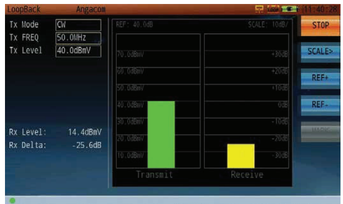
Figure 27: Loopback function is effective for testing attenuation and gain from 5 - 210 MHz. It can measure both CW & QAM signal frequency and sweep frequency.
