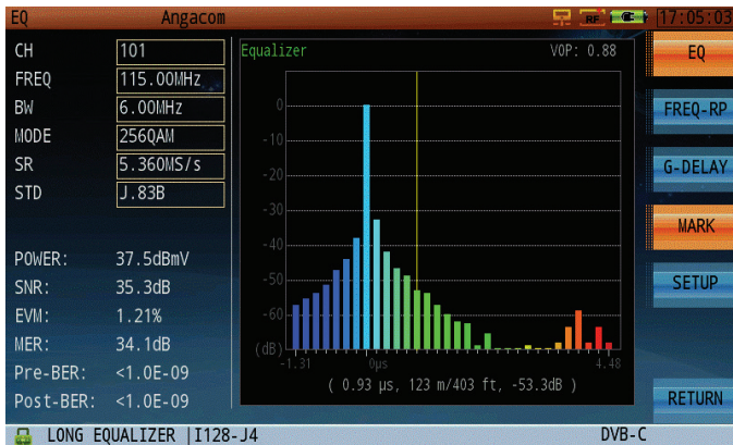
Figure 14: The Adaptive Equalizer uniquely compensates for linear distortions such as phase noise, impedance mismatch & group delay in the HFC network.
