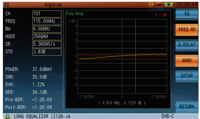
Figure 15: Frequency Response is derived from the adaptive EQ power coefficient. The in-band frequency response should not exceed \pm 1.5 dB peak to valley.
