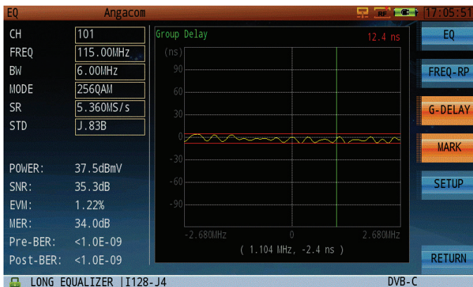
Figure 16: Group Delay is also derived from the adaptive EQ power coefficient. Group delay should not exceed 200 ns/MHz in the US or 75 ns/MHz in the DS.
