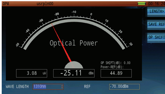
Figure 33: Measure the Optical Power levels at equipment or connector with an easy to interpret graphical gauge.
