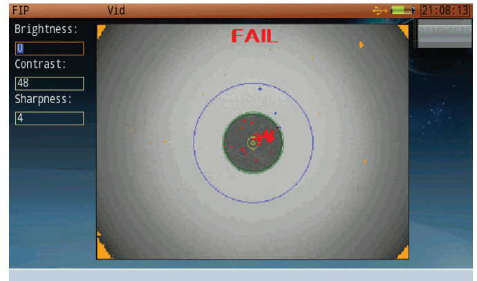
Figure 36: Fiberscope test with dirty connector.
